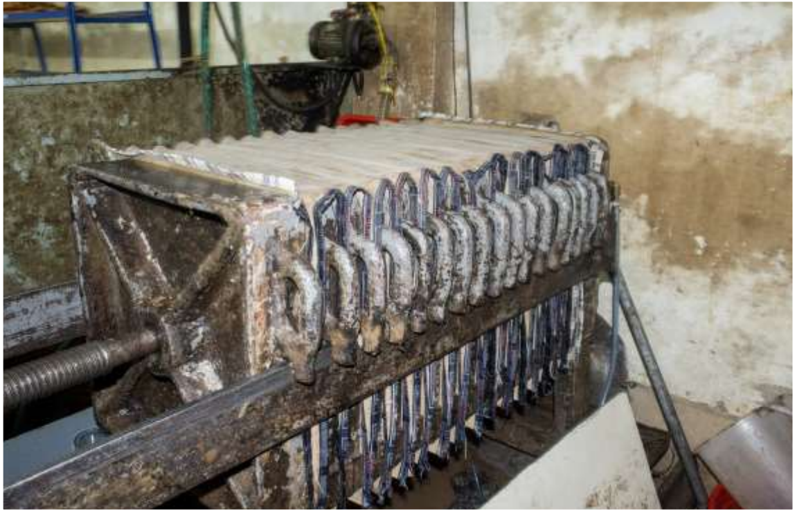
Fig: stacked filters set for filtration of coconut oil
