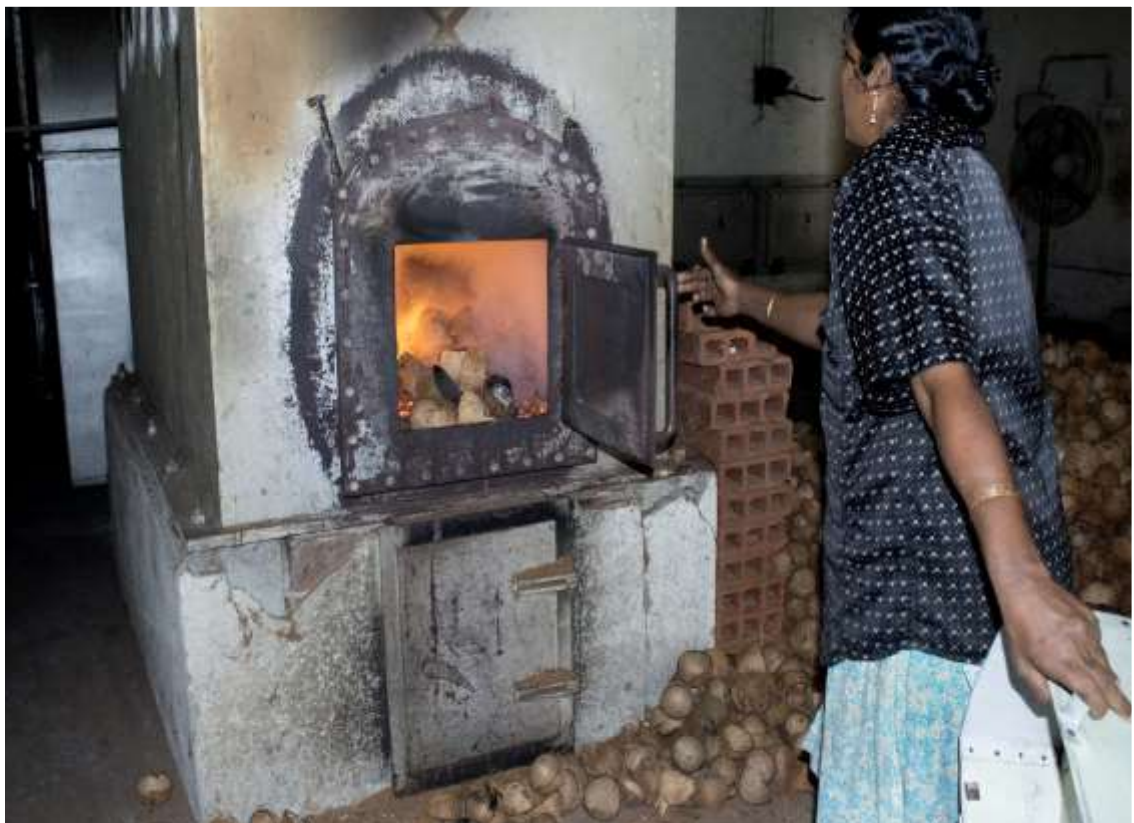
Fig: coconut shells being used as fuel for the hot-air blower
