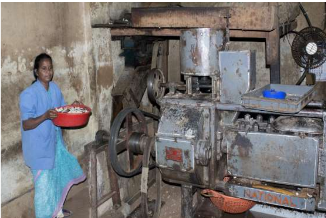
Fig: copra being fed into the expeller
