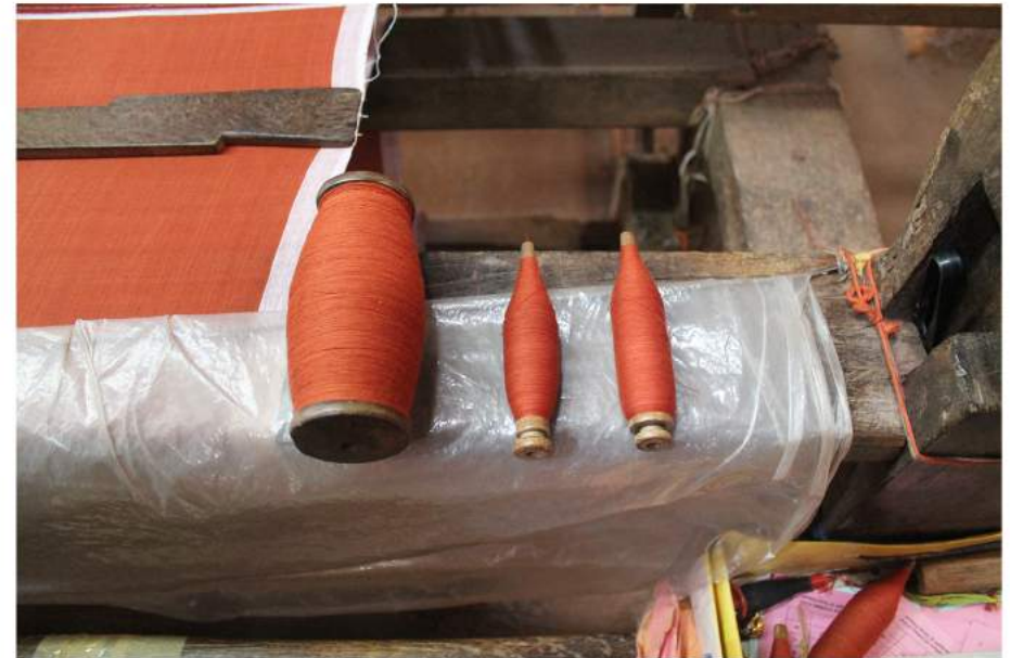
Bobbin on left used for warp and bobbin on right used for weft.
