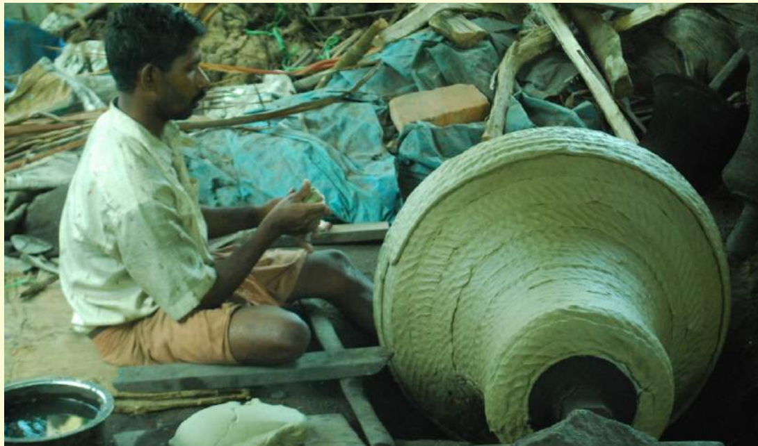
P38. Completing the waxing on a base mould of a bell
