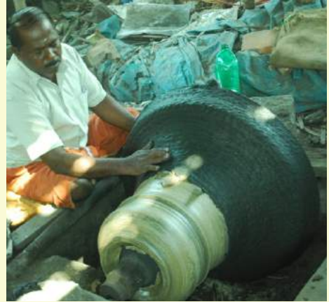
P39. Applying clay layer on waxed mould
