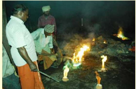
P52. Pouring molten alloy in mould
