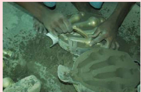
P89 & 90. Sand box mould making
