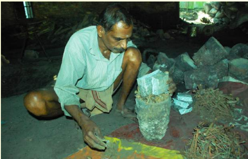
P42. Filling the crucible with weighed metals
