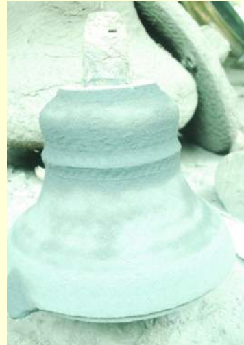
P41. Mould kept in sunlight
