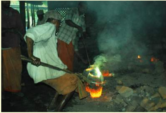
P51. Taking out the crucible
