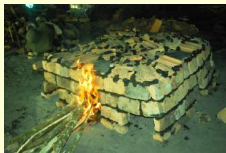
P44. Furnace after ignition
